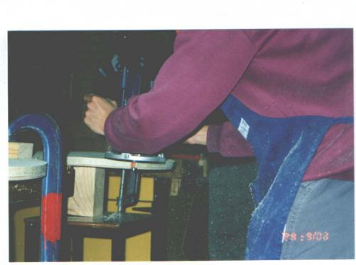
\* Notice the bearing to llow the template underneath the particle board.
